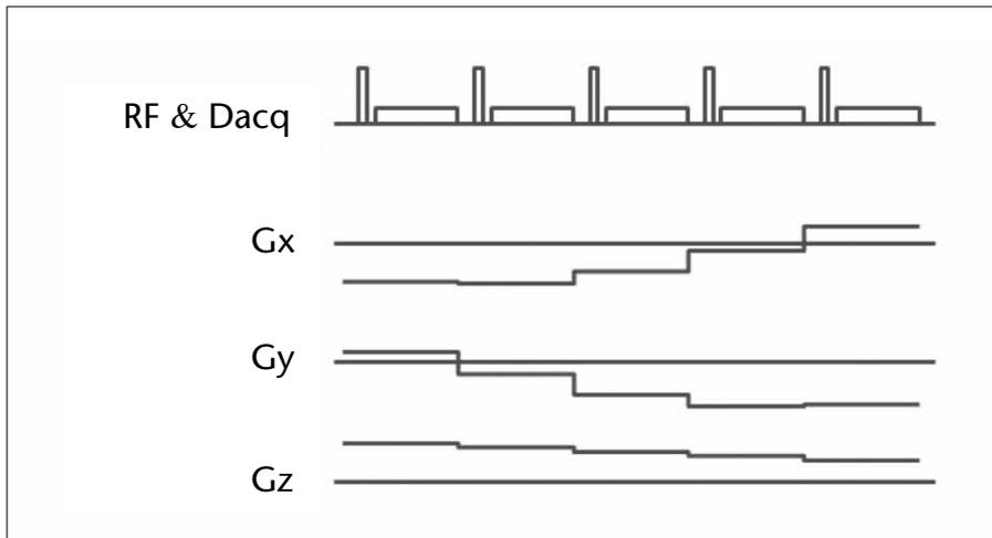
**Figure 1.** Silenz acquisition and k-space readout scheme. Silenz uses a 3D radial center-out data acquisition scheme between radio frequency pulses (RF), stepping through k-space by increasing gradients in small steps. Ramp-up and ramp-down of gradients ( $G_x$ ,  $G_y$ ,  $G_z$ ) between spokes are eliminated, resulting in the silent properties of the pulse sequence.
