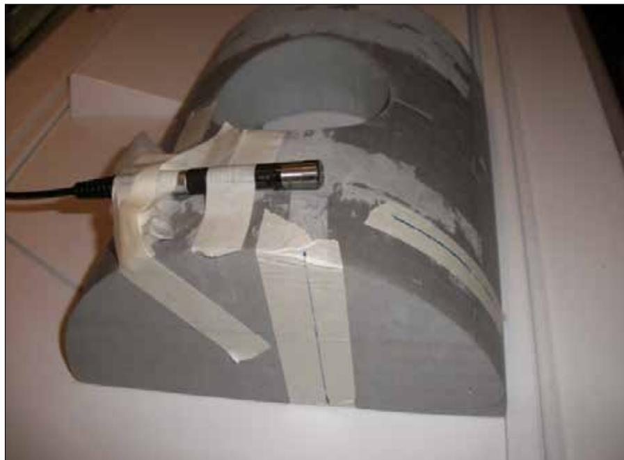
**Figure 2.** The sound level meter is placed in the gantry at a position corresponding to the right ear of the patient.
