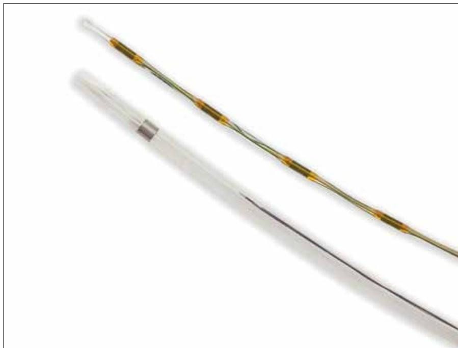
**Figure 1.** The EKOS EkoSonic® Endovascular System consists of a multi-lumen infusion catheter with a removable coaxial US core and a control unit that simultaneously delivers high-frequency, low-energy (2.2 MHz, 0.45 W) US energy and thrombolytic drugs into the thrombus. US exposure enhances the permeability of the thrombus to the lytic agent. The picture of the catheter is courtesy of the EKOS Corporation, Bothell, Washington, USA.
