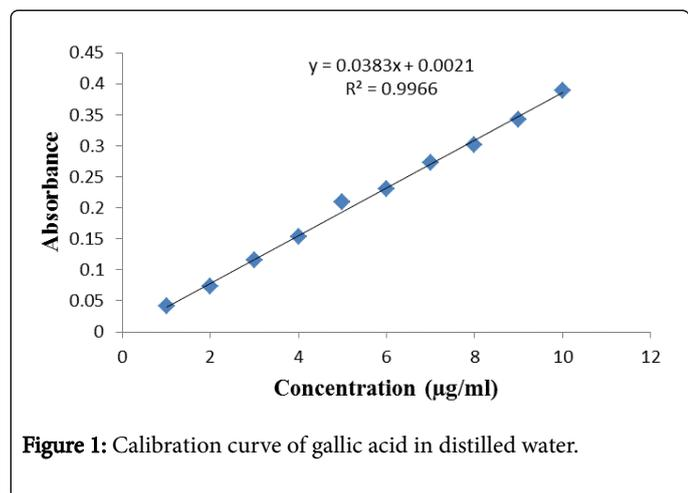
**Figure 1:** Calibration curve of gallic acid in distilled water.
