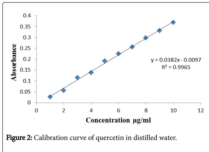
**Figure 2:** Calibration curve of quercetin in distilled water.
